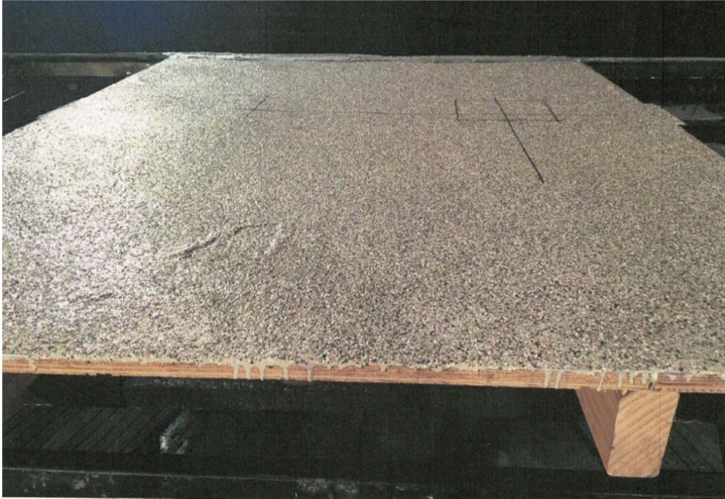
Photograph 1: Class B Burning Brand test Specimen prior to test. Flexstone Pedestrian Deck Coating System
