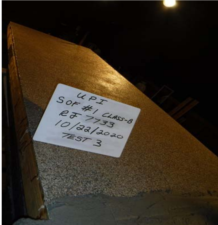
Photograph 1: Class B Spread of Flame test Specimen prior to test. Flexstone Pedestrian deck coating system
