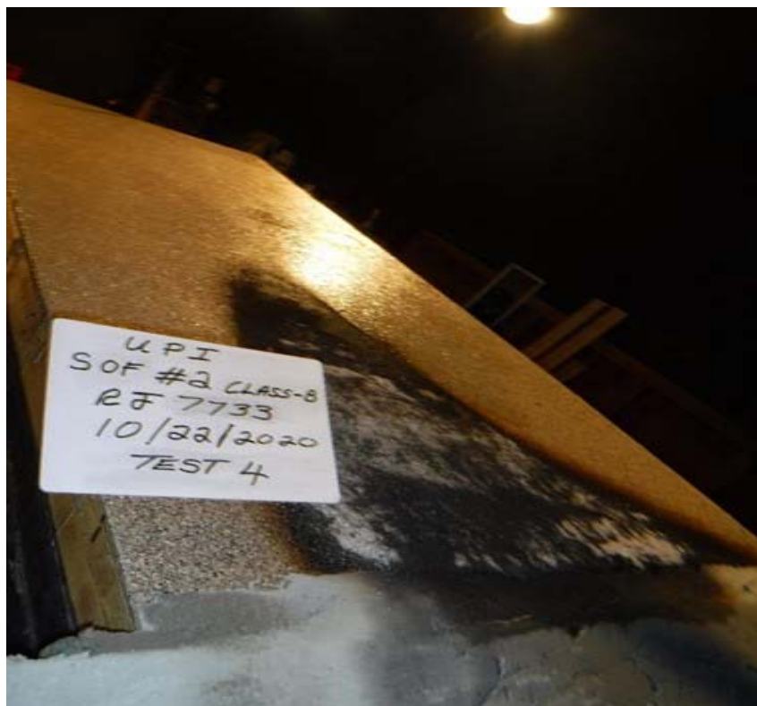
Photograph 4: Class B Spread of Flame after test.
